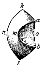
FIG. 153. Space of \gamma solid solution between the sections shown in Figs. 151 and 152.
